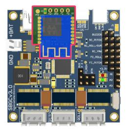
Option2: connect by cable to the UART or RC\_SERIAL port
