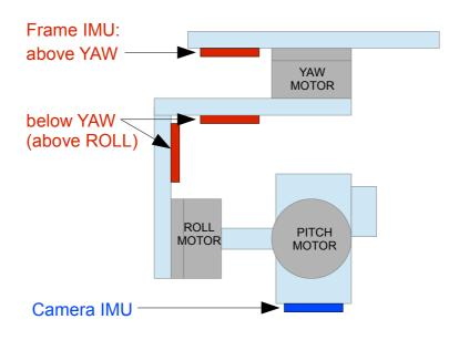
If the sensor is placed above YAW motor, it helps to stabilize ROLL, PITCH and YAW motors. But the system becomes less stable during long work (because the frame heading, estimated from the second IMU, may drift with time and auto-correction may not work in all cases).
