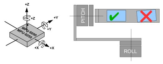
Skip Gyro calibration at startup - With this option, the board starts working immediately after powering it on, using the saved calibration data from last gyroscope calibration call. However, stored calibration data may become inaccurate over time or during temperature changes. We recommend you to re-calibrate your gyro from time to time to ensure the best performance.
