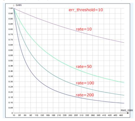
• Recovery factor, 0..10 - defines, how fast PID gains are recovered back when the system becomes stable. Too low of a value may increase a chance that vibration comes back in a short time. Too high of a value may cause worsen of operation (because lowered PID values are kept longer). Recommended value is 5..6
