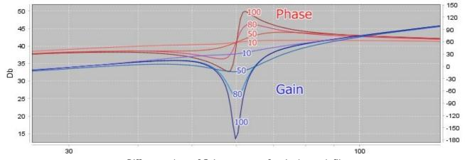
Different values of Gain parameter for single notch filter
