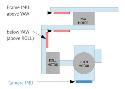
If the sensor is placed **above YAW** motor, it helps to stabilize ROLL, PITCH and YAW motors. But the system becomes less stable during long work (because the frame heading, estimated from the second IMU, may drift with time and auto-correction may not work in all cases).
