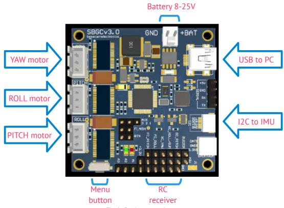
Fig.1 Basic connections
