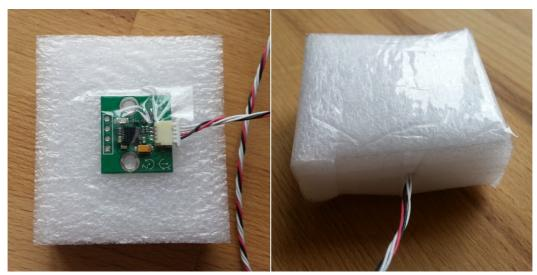
Thermal insulation of the sensor
