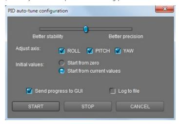
The slider at the top defines the target of tuning. If its close to "Better precision", it will try to achieve maximum gain and keep it. If close to "better stability", it will find maximum gain and then decrease it by 30-50% to make the system more stable.
