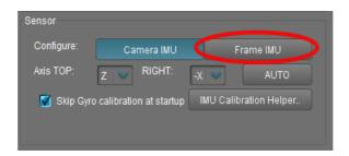
If the second IMU is connected properly, this button becomes active. After pressing on it, all IMU settings now affect the frame IMU. You may notice the right panels with arrows are displaying now angles not for the main, but rather for the frame IMU. Also, in the "Monitoring" tab, accelerometer's and gyroscope's data are for the frame IMU.
