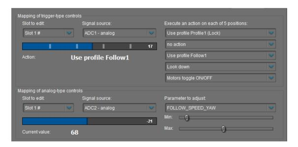
There are two types of control: Trigger and Analog.
